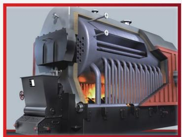
Solid fuel fired boiler consist of two parts, water-tube and fire- tube type boilers in a single united body. Primary furnace as water- tube (tube+bar) boiler mounted on a rotating grid is manufactured as high enough height to from a large volume of combustion chamber on the grill. Scotch type fire-fume tube type boiler and flame radiation type water tube boiler are connected to each other by means of water collector.
